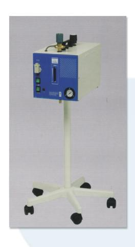
industrial steam generator with round boiler 5 Liters, pressure switch for exact control of steam pressure, visual control of the waterline in the boiler, ball valve for deposit and water outlet, steam valve with control of steam flow, safety valve cap, No. 02 safety thermostats to protect the heating elements in case of lack of water and to protect the boiler against too high temperature s.
